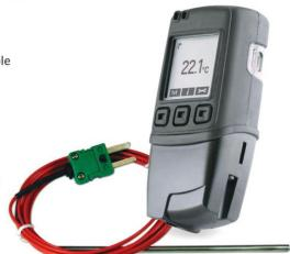
This standalone data logger measures and stores more than 250,000 temperature readings from a K, J or T-type thermocouple at a resolution of 0.1°C (0.2°F). It comes supplied with a K-type thermocouple capable of measuring from 0 to 200°C (32 to 392°F).
